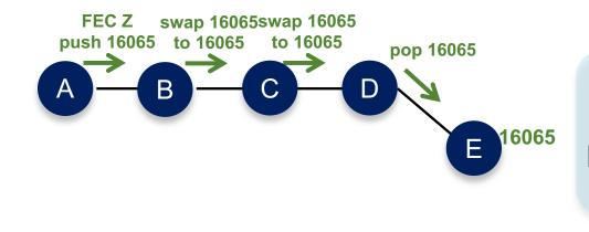
A packet injected anywhere with top label 16065 will reach E via shortest-path
