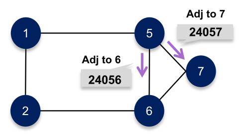
A packet injected at node 5 with label 24056 is forced through datalink 5-6
