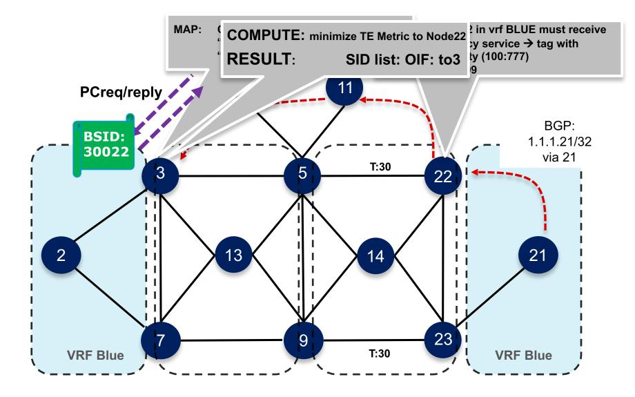
Automated Steering uses color extended communities and nexthop to match with the color and end-point of an SR Policy E.g. BGP route 2/8 with nexthop 1.1.1.1 and color 100 will be steered into an SR Policy with color 100 and end-point 1.1.1.1 If no such SR Policy exists, it can be instantiated automatically (ODN)
