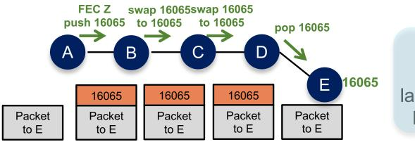
A packet injected anywhere with top label 16065 will reach E via shortest-path
