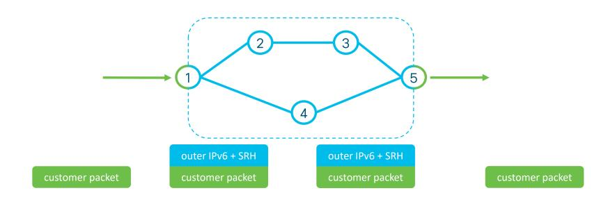
• Egress PE removes the outer IPv6 header as the packet leaves the SR domain
